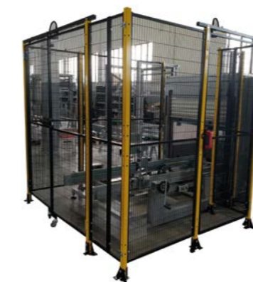
Fig. 11 Perimetral safety protections CAR
